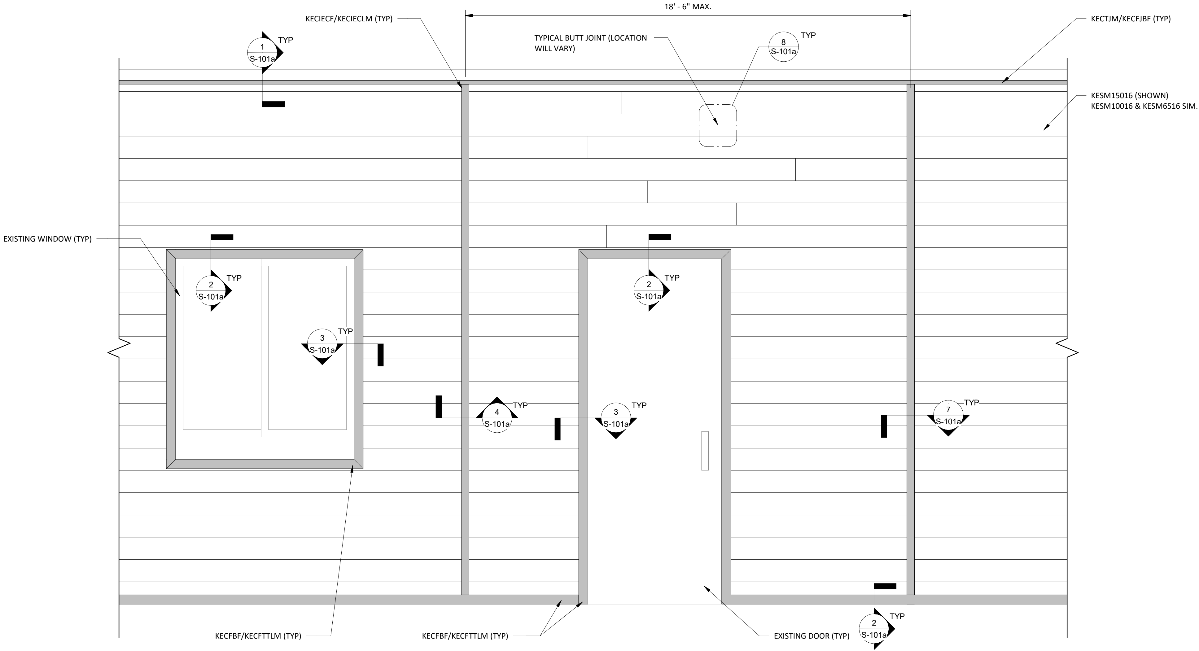
2 HORIZONTAL CLADDING GENERIC ELEVATION VIEW 3/4" = 1'-0"
