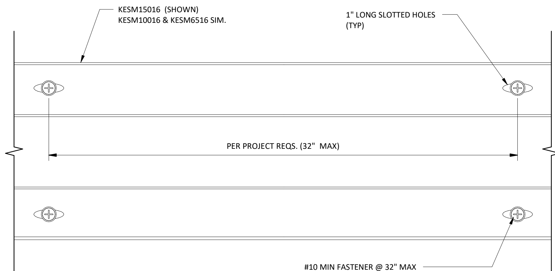
9 TYPICAL SLOTTED HORIZONTAL CLADDING CONNECTION DETAIL 6" = 1'-0"
