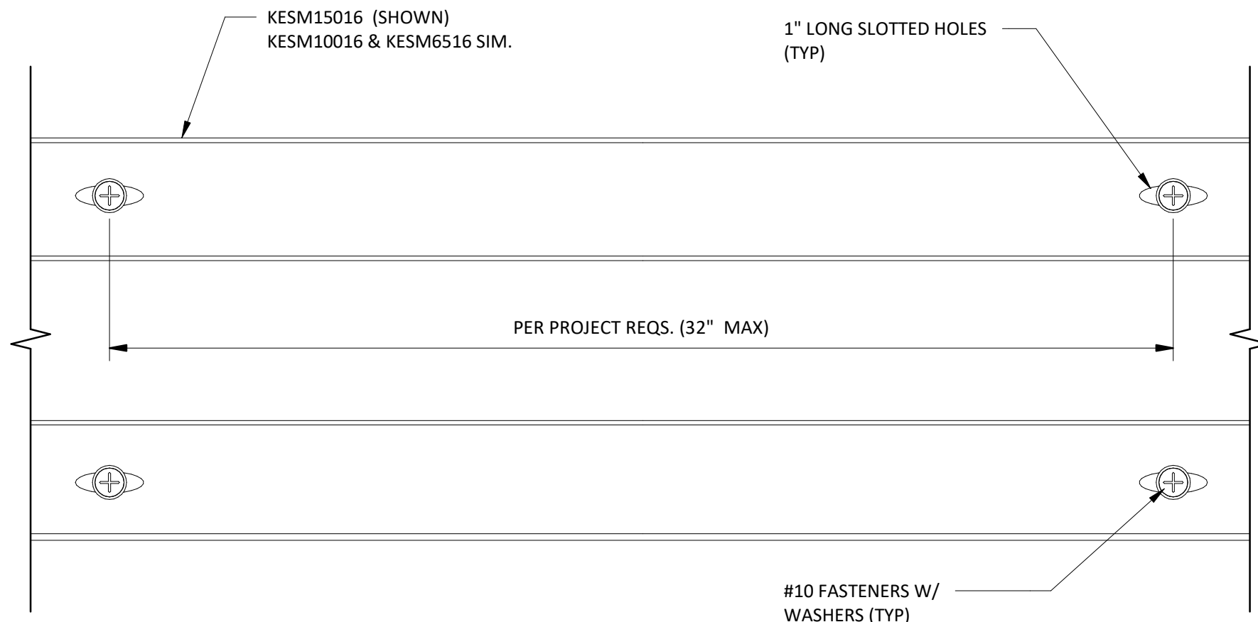
9 TYPICAL SLOTTED CLADDING TO LG CONNECTION DETAIL 6" = 1'-0"
