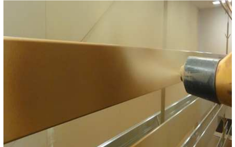
Powder coating on aluminum is a minimal maintenance solution as it is easy to clean and maintain.
