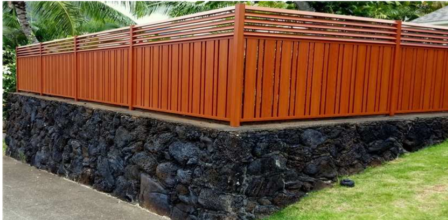
Vertical fence with alternating 6" and 2" slats with spacer mounted on traditional Hawaiian rock wall with added privacy louvers
