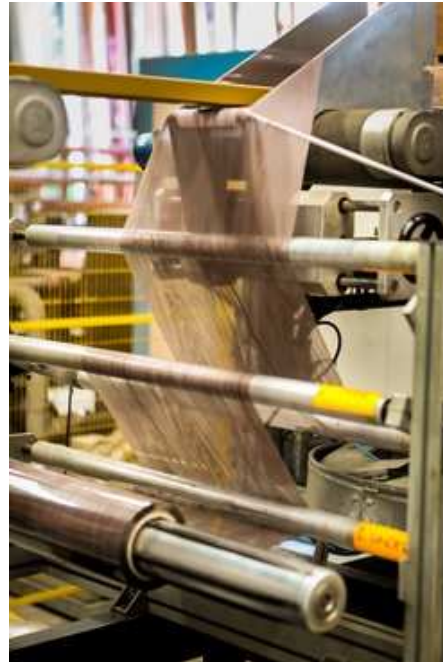
The process of art sublimation ensures the wood-grain film covers the entire aluminum profile.
